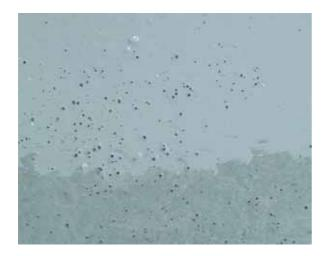
Defective pore sealing due to lack of primer
