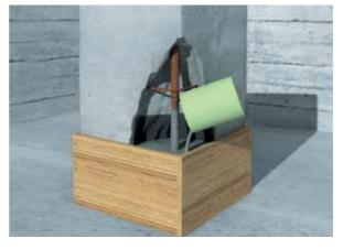
Repairs using fluid mortar
